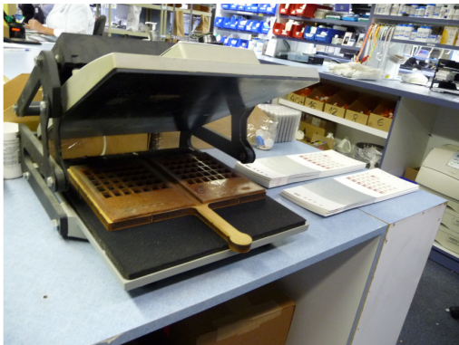
Figure 11: Heat sealer for blister cards
